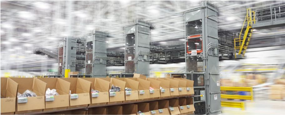
The vertical conveyor was designed to raise and lower product, where floor space is restricted. **JMP Solutions' continuous vertical conveyors** are designed to accept product horizontally, convey it vertically, and discharge it horizontally; all in one continuous non-stop operation. An in feed belt synchronized with the vertical conveyor, loads product into the lift; operator supervision is not required.
