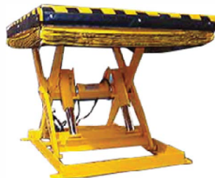
SLS with safety enclosure and painted Safety Yellow
